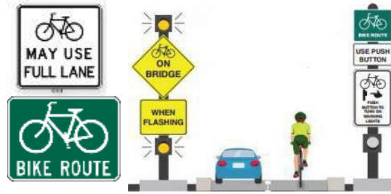
"Bikes on Bridge" activated warning.
