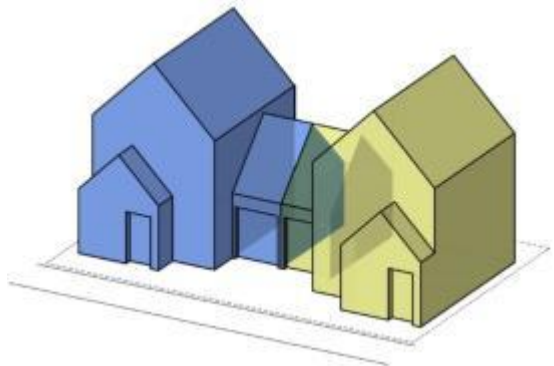
Duplex attached by a breezeway
