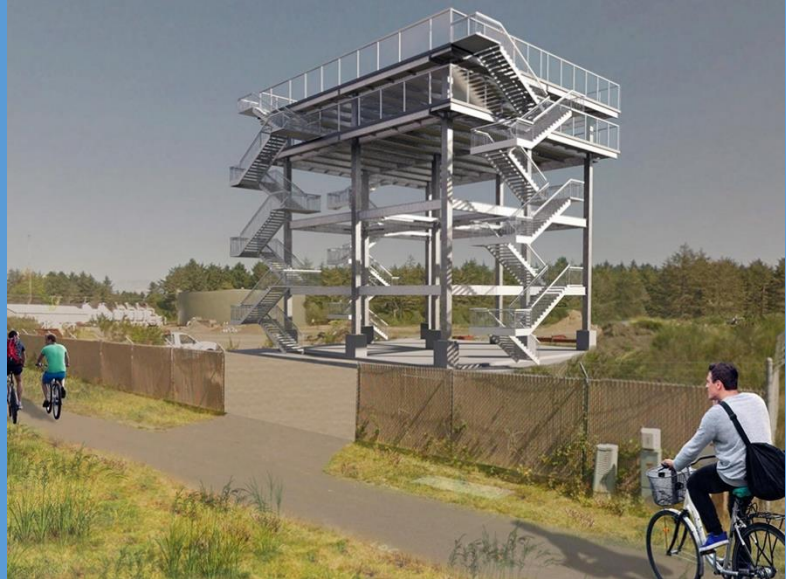
Figure 25 Tsunami Escape Tower Example, Tokeland, WA Source: Degenkolb conceptual design for FEMA grant application.
